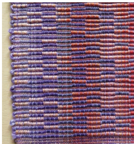
24 shaft Repp designed by my Master Class students, Marilyn Burton: 20/2 Mercerised Cotton in the warp sett at 60 ends per inch (24 ends per cm).
